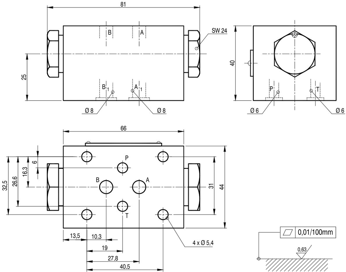
Admissible surface roughness and flatness deviation for a subplate face.
